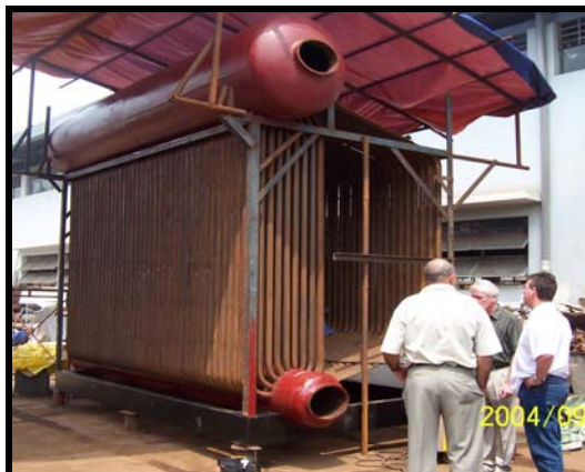
Thermic's Boiler production inspected and witness by external inspector.
